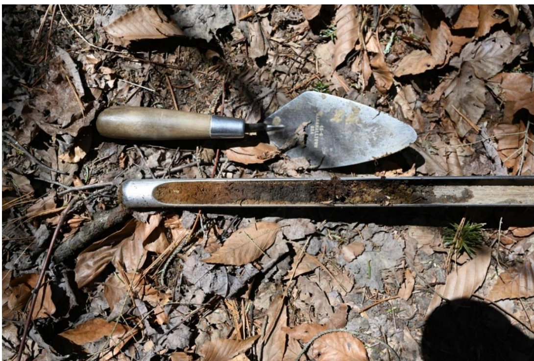
Figure 20. View of a hand core showing a largely undisturbed upper soil profile in the archaeologically sensitive area within the western access route on the right (west) side of the impoundment.
